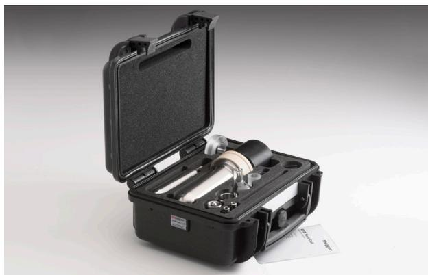
OTD Test Cell in a toughened transport case. Provided as standard with the OTD instrument. This test cell contains 32 components making it easy to clean and assemble.
