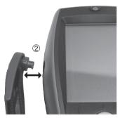
1 Remove sealing caps from the sides of the housing.
