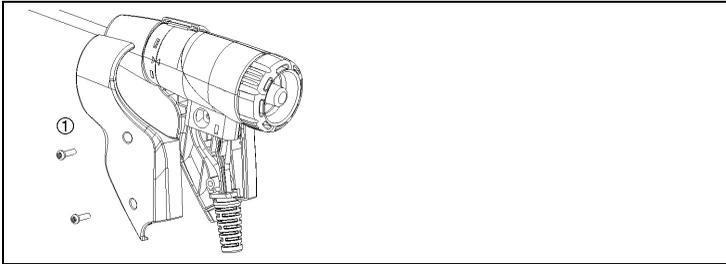
1. Loosen and remove halfshell handles (1).
