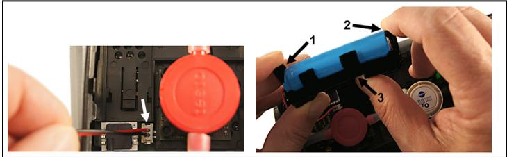
4. Unplug the plug-in connection from the slot.
