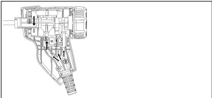
6. Connect the adapter and hose to the thermocouple (8). Adjust cables and hoses (9), refit halfshell elements.
