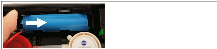
8. Insert the holder into the guide rail and slide it in the direction of the arrow until the holder clicks into place.
