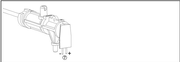
5. Connect cables to the new thermocouple (white -, green +) (7) and push the thermocouple back into the holder.
