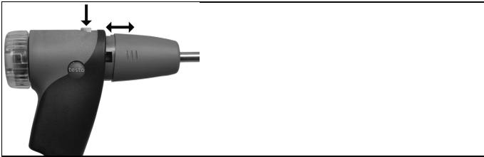
1. Release the probe catch by pressing the key on the probe handle and remove the probe module.
