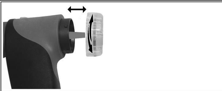
1. Open the filter chamber: turn slightly anti-clockwise.
