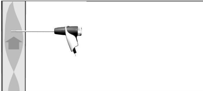
The tip of the probe must be in the centre of the flue gas flow.
