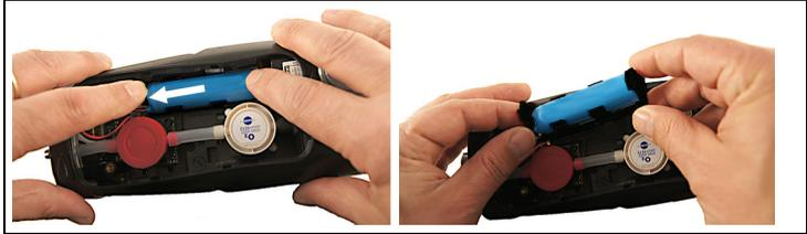
3. Press down on the holder lightly with your fingers. Pull the retaining clip in the direction of the arrow until the catch is released. Remove holder.
