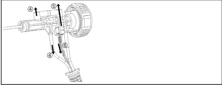
4. Remove the adapter (4) and hose (5), push the thermocouple out of its holder and disconnect the cable (6) from the thermocouple.
