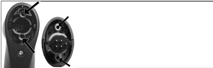
2. Blow compressed air through the flue gas ducts in probe module and probe handle (see illustration). Do not use a brush!
