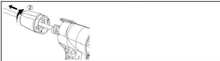
2. Turn the sealing cap (2) clockwise as far as it will go and remove probe shaft.
