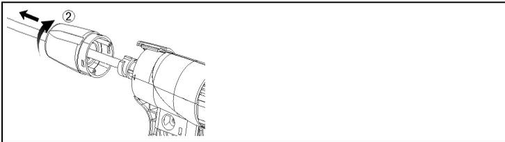
2. Turn the sealing cap (2) clockwise as far as it will go and remove probe shaft.
