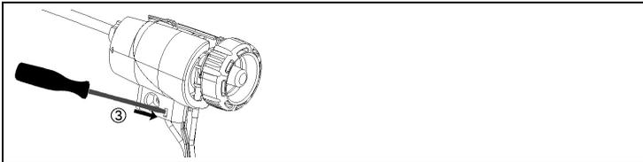
3. Release halfshell elements (3) and remove.
