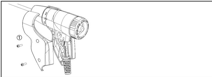
1. Loosen and remove halfshell handles (1).
