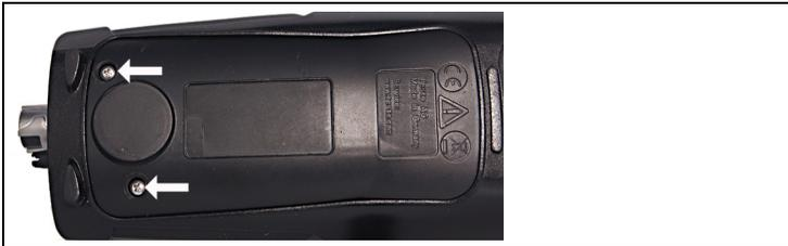
2. Unscrew, lift up and remove the service cover.
