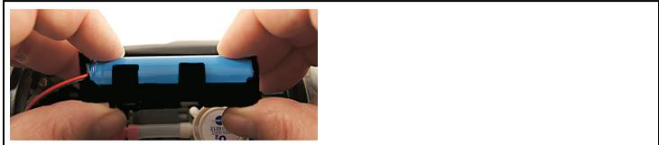
6. Insert the new rechargeable battery in the holder. Make sure that the plug-in connection cable is routed out of the holder at the side. Press the rechargeable battery into the holder until the retaining clips click into place.
