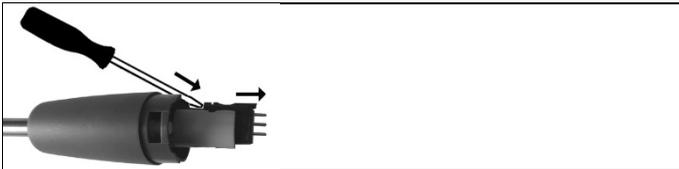
2. Remove the thermocouple plug-in head from the socket using a screwdriver and pull the thermocouple out of the probe shaft.
