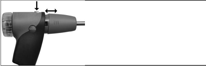
1. Press the key on the top of the probe handle and remove the probe module.
