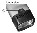
**E1**: Front bezel is not fastened correctly. If the E1 message appears, the instrument must be switched off. Remove the front bezel screw, reseat the reflector and tighten the front bezel screw (①).
