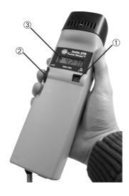
The **testo 476** can be operated with and without mains unit. The Lithium ion rechargeable battery is recharged when the instrument is connected to the mains unit.
