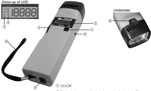
② Flash Adjustment Knob adjusts the flash rate. The speed with which the flash rate changes is controlled by how quickly the knob is rotated:
