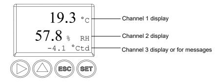
Four keys enable the user to navigate/scroll through the menus and enter/amend values and settings:
