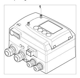
1 Loosen screw connection (1) of service flap and open the flap.
