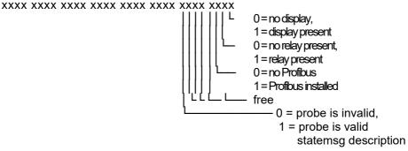
Content of statemsg is a double word type number (32 bit). The individual status messages are bit-coded here.
