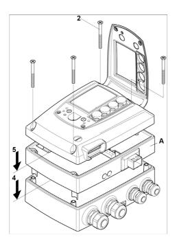
4 Place Ethernet module (A) on lower part of instrument (4).
