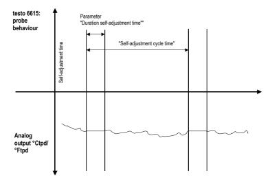
The heating time and storing of cycles can be edited in the P2A software; for example, they can be deactivated by setting the two parameters to "0".
