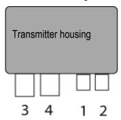
Plug-in connections for power supply and channels M12 plug-in connection (5-pin) socket (1)
