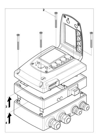
2 Loosen and remove housing screws (2).
